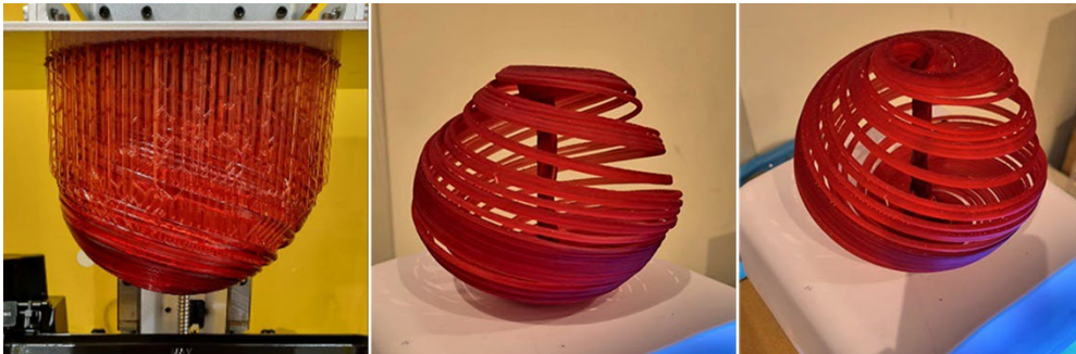
Fig 4. Fabricating a strange attractor with a 3D printer
