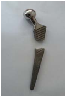
Fig. 2. Broken extracted femoral stem.
