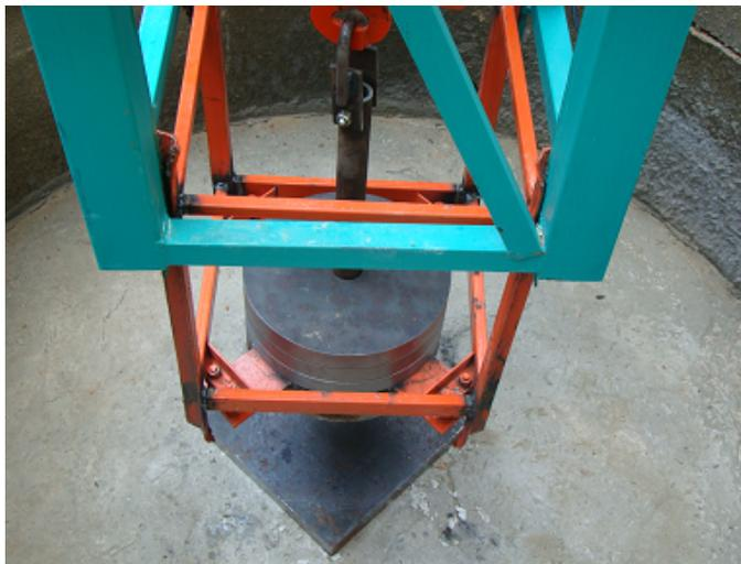
Fig. 2: The guiding system, the weight and the anvil.
