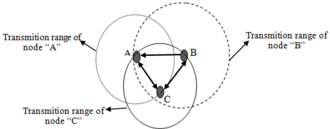
In unidirectional BA link, node B is upstream node and node A is downstream node.
