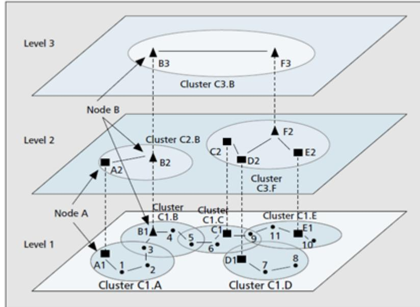
Node B has three wireless interfaces and works as cluster head in all levels. C1.A means that node A is the cluster head of c1 cluster, which is in level one.
