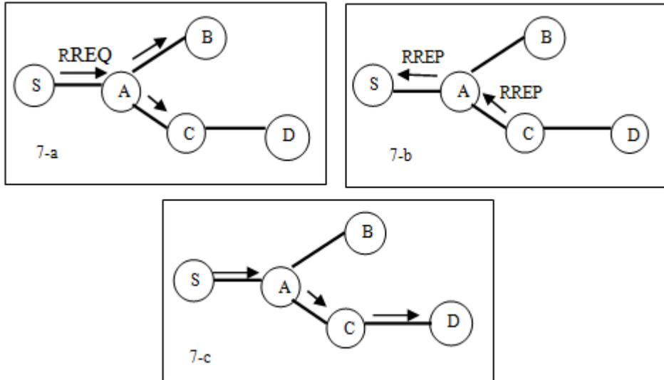
Figure 7: Route discovery and Packet sent in AODV
