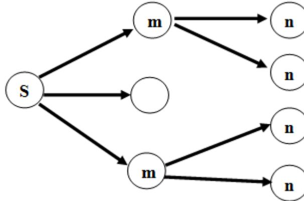
The nodes labeled as (m) are MPRs of the node labeled as (s). Node s can communicate with nodes n by its MPRs (nodes m).
