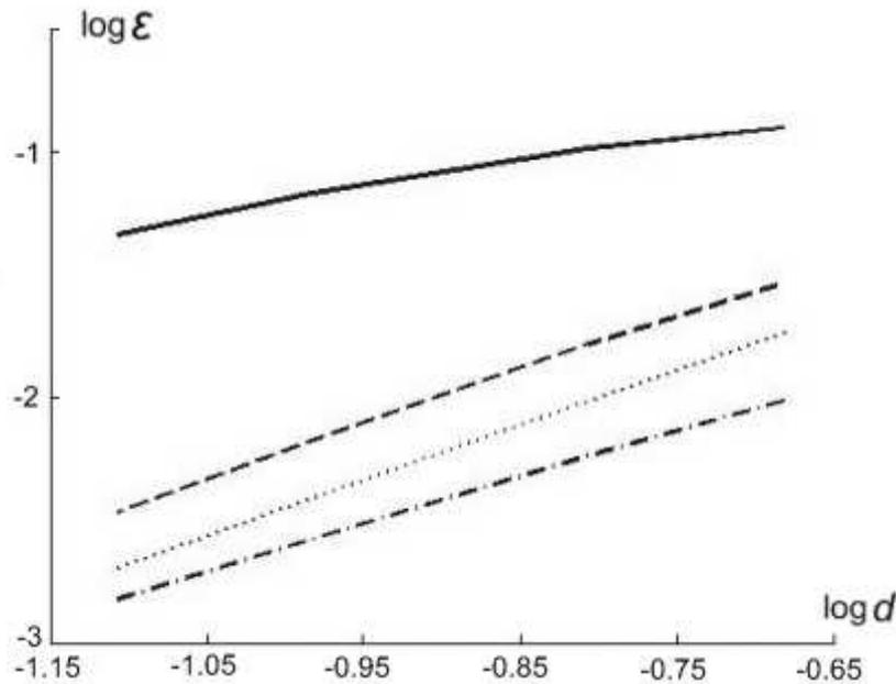
Figure 2: Error norm via the grid resolution in logarithmic scale for  $L_2$ -error: solid line—pressure, dashed line  $-v_r$ , dotted line  $-v_\theta$ , dash-dot line  $-v_\phi$ .
