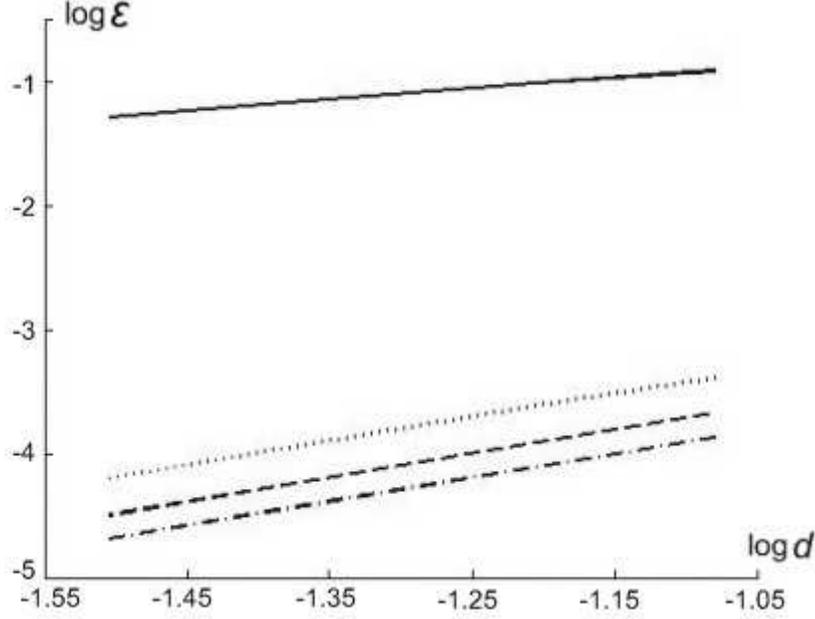
Figure 1: Error norm via the grid resolution in logarithmic scale for  $L_2$ -error: solid line- pressure, dashed line-  $v_r$ , dotted line-  $v_\phi$ , dash-dot line-  $v_z$ .
