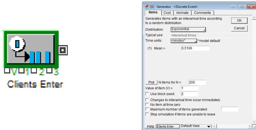
Figure 7. Block Generator and the setting of its parameters
