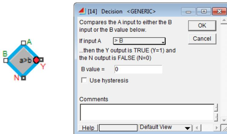
Figure 11. Block Decision and the formation of a rule for comparing the input parameters
