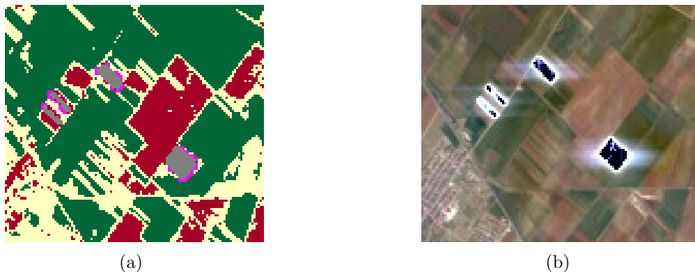
Figure 8: a) The anomalies in the NDVI; b) color RGB composite of the PRISMA image section containing the solar panels.
