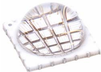
Fig. 5. LED with multi-layer ceramic substrate [6]
