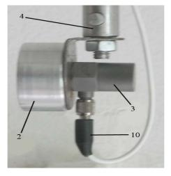
Fig. 2. *The accelerometer fixed on the impact body* 2 – impact body, 3 – accelerometer, 4 – the pendulum arm; 10 – signal cable
