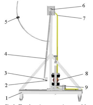
Fig. 1. *The schematic representation on pendulum* 1- mainframe; 2 - impact body; 3-accelerometer; 4 – pendulum arm; 5- electromagnetic device;6 – rotary encoder; 7- electrical connector; 8 – potato; 9 - sample holding system.
