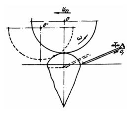
Fig. 5. Trajectory of the cutter cutting beet head
