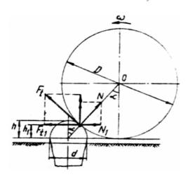
Fig. 3. Correlation scheme between palpator diameter and the beet head dimensions
