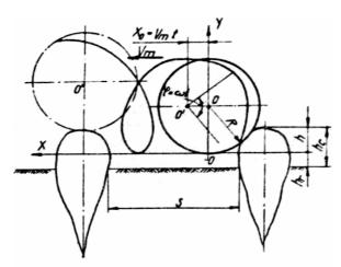
Fig. 1. Scheme of the cylindrical palpator kinematics of sugar beet head cutting equipment
