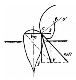
Fig. 2. Scheme of movement coordination between palpator and machine
