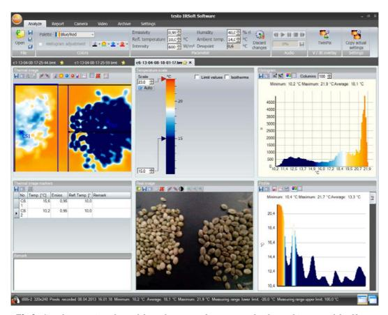
Fig.2. Graphic user interface of the software used to process the thermal images of the fiber hemp seeds.
