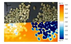
Fig.1. Illustration of the seed samples exposed against the thermal background used for determination of the quality of fiber hemp seeds using the thermo-camera.
