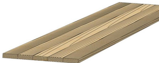
Fig. 6. Predicted appearance of the panel glued sequentially edge-to-edge from pieces of lumber No s 1-5
