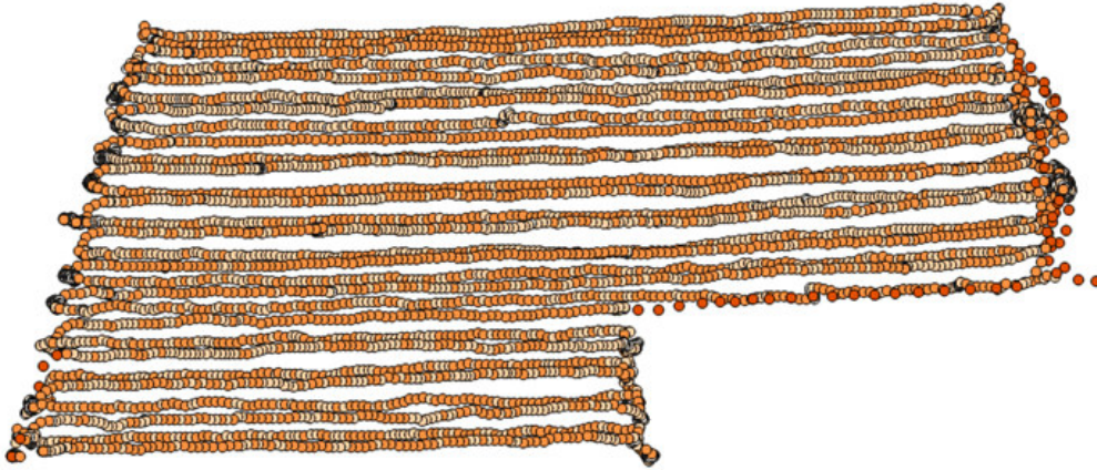
Fig. 3. GPS speed classification in QGIS based on data from D1: an example for a planted plot using natural breaks as a classification rule. Note: the map is rotated 90 degrees to the right
