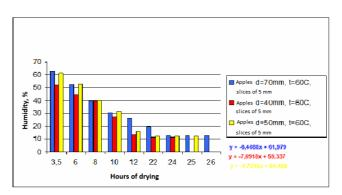
Fig. 14. The influence of the initial dimension of the sample on drying duration in the case of apples slices of 5mm thickness, dried at a temperature of 60°C
