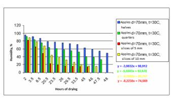
Fig. 13. The influence of the system of slicing on the drying time in the case of apples with a diameter of 70mm dried at a temperature of 30°C
