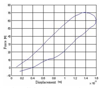
Fig. 3. Theoretical curves of the force-deformation variation in the impact area for potato tubers
