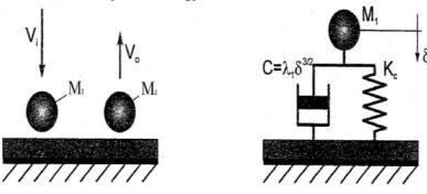
Fig. 1. *The impact pair model [4]: a – impact model; b – elastic equivalent model*
