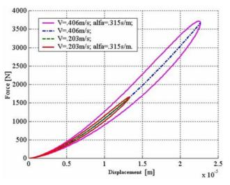
Fig. 2. Force variation (elastic and total component) upon impact depending on penetration in the contact area (Hunt and Crossley) [4]
