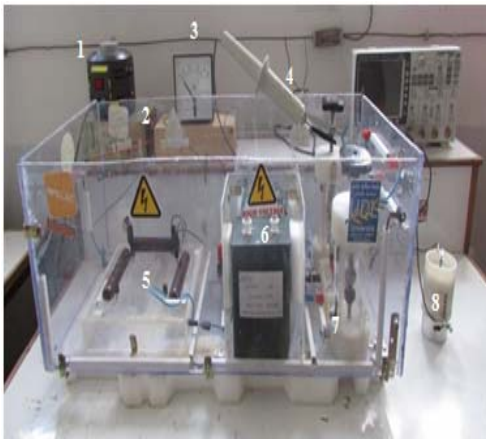
Fig. 4. The experimental set-up: Auto-transformer - (2) HV DC power supply - (3) Electrostatic voltmeter - (4) HV measuring probe - (5) Charging resistors - (6) HV charging capacitor - (7) spark-gap discharger - (8) Treatment chamber
