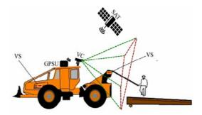
Fig. 1. A concept of equipping a winch skidder with external sensors able to automatically collect production data: SAT - satellite, GPSU - GPS unit, VC - digital video camera, VS - vibration (motion detection) sensor
