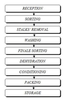
Fig. 1. The Scheme of the techprocess of the berries' dehydration by convection
