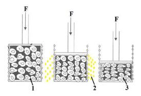
Fig. 1. Schematic representation of the pressing process (hydraulic presses): F – pressing force, 1 – raw material, 2 – crude oil press, 3 – press cake
