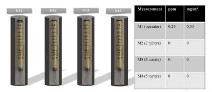
Fig. 4. Ammonia emission measurements, with the revised version of the emulsion preparation system
