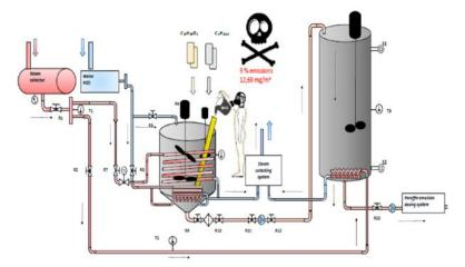
Fig. 1. In-line paraffin emulsion preparation system, 1<sup>st</sup> version (original)
