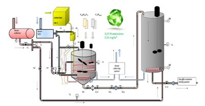
Fig. 3. In-line paraffin emulsion preparation system, revised version (original)
