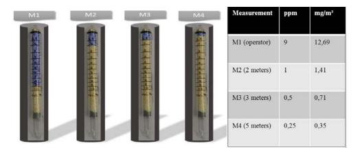
Fig. 2. Ammonia emission measurements, with 1<sup>st</sup> version of emulsion preparation system
