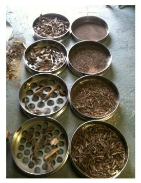
Fig. 1. Sieves used in fractioning out the particle sizes of the hogfuel
