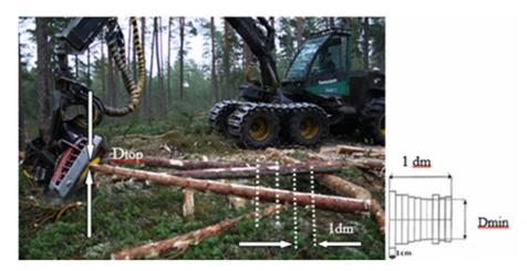
Fig. 1. Example of Timbermatic principles of controlling head diameter measuring, where  $D_{min} \ge D_{top}$
