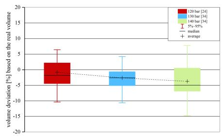
Fig. 4. Volume deviation as a result of increasing roller pressure
