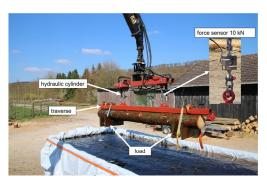
Fig. 2. Image of water immersion process
