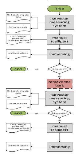
Fig. 1. Measurement sequence of comparative measurements
