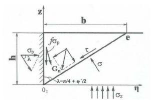
Fig. 2. Inclination of the movement plan (3)
