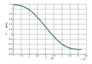
Fig.2. The impact velocity evolution in time
