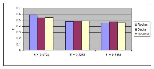
Fig. 3. The comparative graph of restitution coefficient variation for three impact energies
