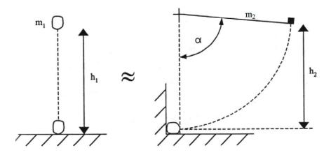
Fig. 1. Testing the potato tubers with pendulum device [3]
