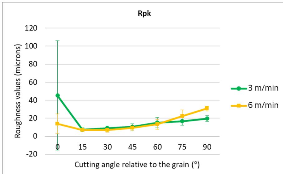
Fig. 10. The variation  $R_{pk}$  with cutting angle and feed speed
