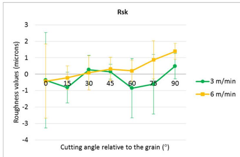
Fig. 13. The mean values of the  $R_{sk}$  parameter, CNC routed with two feed speeds and seven cutting angles relative to the grain evaluated for beech surface
