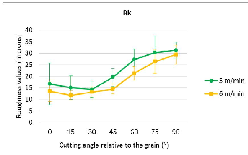
Fig. 9. The variation of the processing roughness  $R_k$  with cutting angle and feed speed
