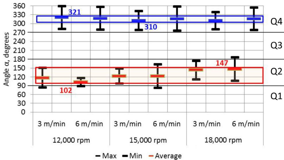
Fig. 7. Graphic representation of the limits and mean values of the central angles for which defective surfaces affected by machining have been observed
