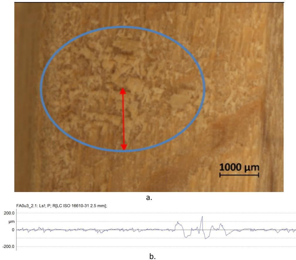
Fig. 11. Microscopic images of the processed flank-a- (30x magnification) and roughness profile measured from the same surface-b- (red arrow indicates the measuring line) processed at  $0^\circ$  angle. Raised fibres area (blue ellipse)
