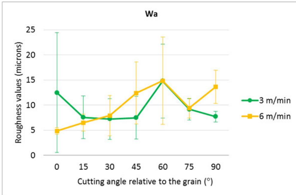
Fig. 16. The mean values of the  $W_a$  parameter, CNC routed with two feed speeds and seven cutting angles relative to the grain evaluated for beech surface
