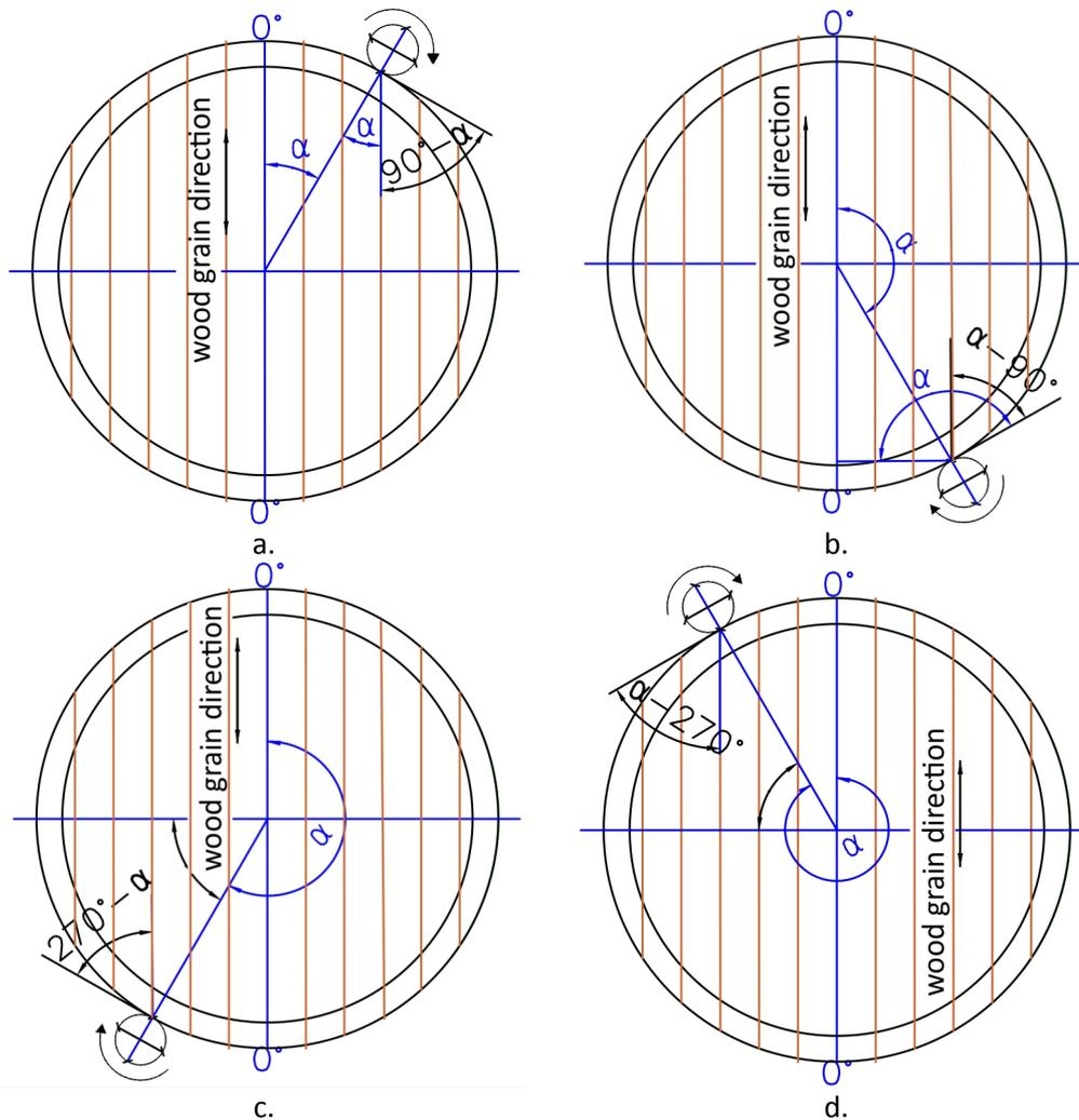
Fig. 2. Calculation of milling angle relative to grain direction, based on the central angle of the circle,  $\alpha$ : a - for quadrant 1 ( $Q_1$ ); b - for quadrant 2 ( $Q_2$ ); c - for quadrant 3 ( $Q_3$ ); d - for quadrant 4 ( $Q_4$ )
