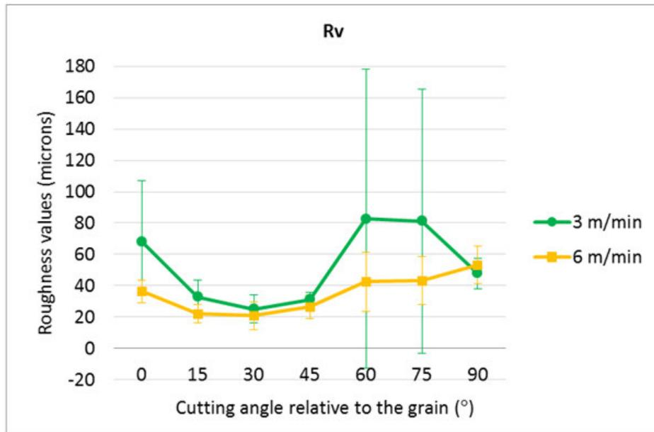
Fig. 14. The mean values of the  $R_v$  parameter, CNC routed with two feed speeds and seven cutting angles relative to the grain evaluated for beech surface
