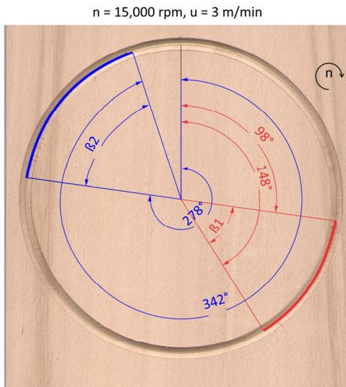
Fig. 3. Scanned image of one beech panel and the circle machined by CNC on the wood surface with highlighting of the visible areas where machining defects occur
