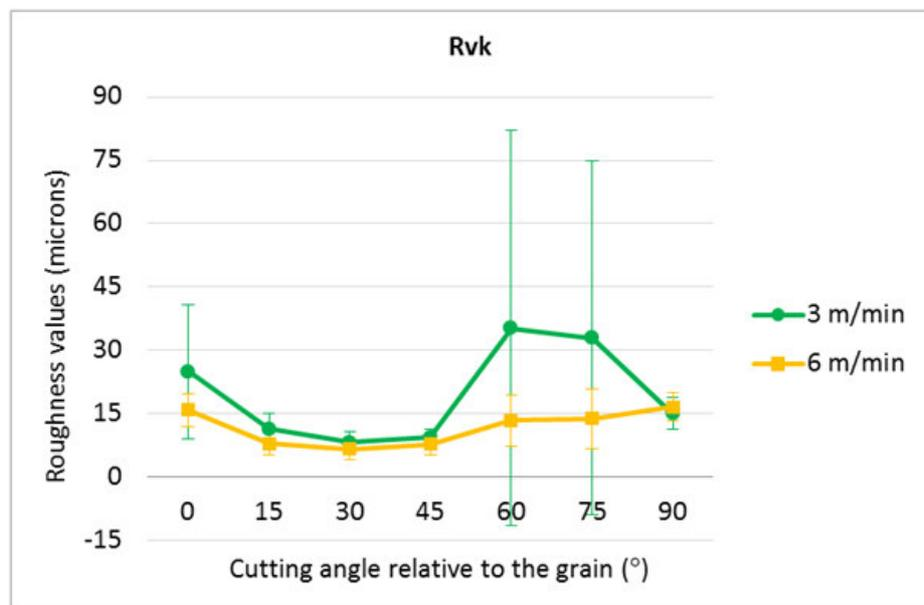
Fig. 15. The mean values of the  $R_{vk}$  parameter, CNC routed with two feed speeds and seven cutting angles relative to the grain evaluated for beech surface
