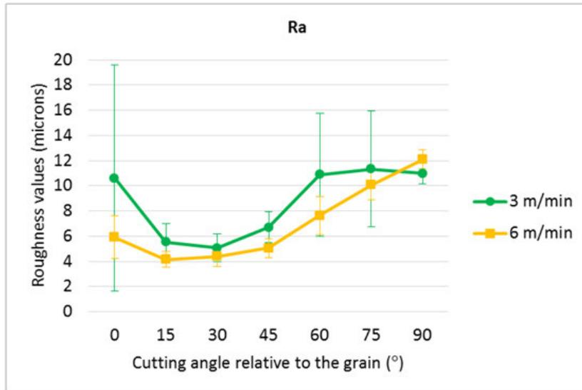
Fig. 12. The mean values of the  $R_a$  parameter, CNC routed with two feed speeds and seven cutting angles relative to the grain orientation evaluated for beech surface
