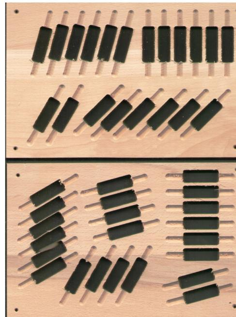
Fig. 4. The panels from which the samples for roughness measurement were cut
