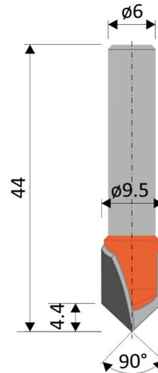
Fig. 1. The CMT Orange V-groove router bit with a 90° angle used in milling on solid wood panels
