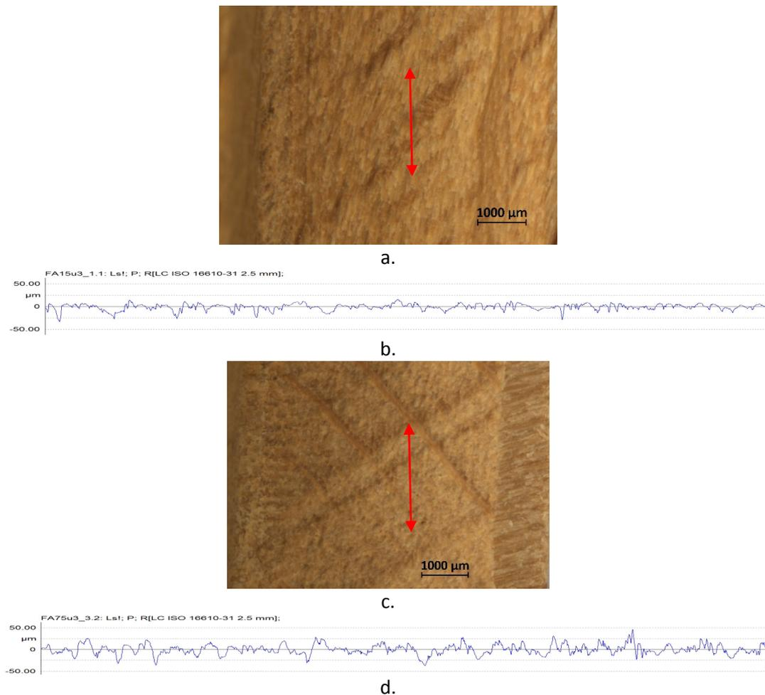
Fig. 8. *Microscopic images of the processed flank-  $u=3$  m/min- (30x magnification) and roughness profile measured from the same surface (red arrow indicates the measuring line); a. and b. 15° cutting angle; c. and d. 75° angle*
