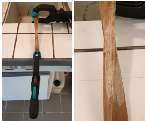
Fig. 2. Examples of bent wood artefacts made by plasticizing wood with ammonia solution
