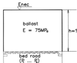
Fig. 4. *The reduced road system, composed of a ballast layer, situated on the base*
