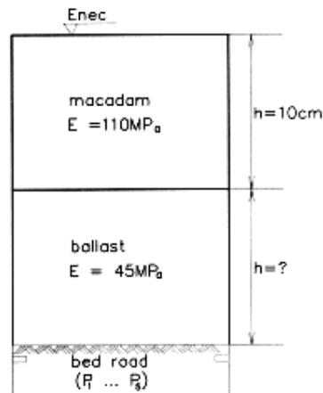
Fig. 5. The road system composed of two layers, clothing of macadam and foundation of ballast
