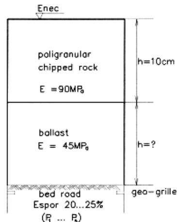
Fig. 3. *Two-layered road system of polygranular chipped stone and ballast on geo-textile*
