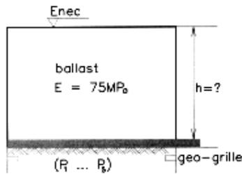
Fig. 1. *One-layered road system from ballast on the geogrid*
