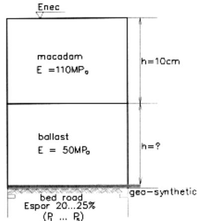
Fig. 2. *Two-layered road system of macadam and ballast over geo-textile*
