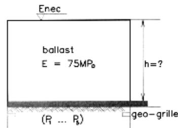
Fig. 6. The road system composed of a traffic layer and a ballast wear layer placed on a geo-grille situated on the way bed
