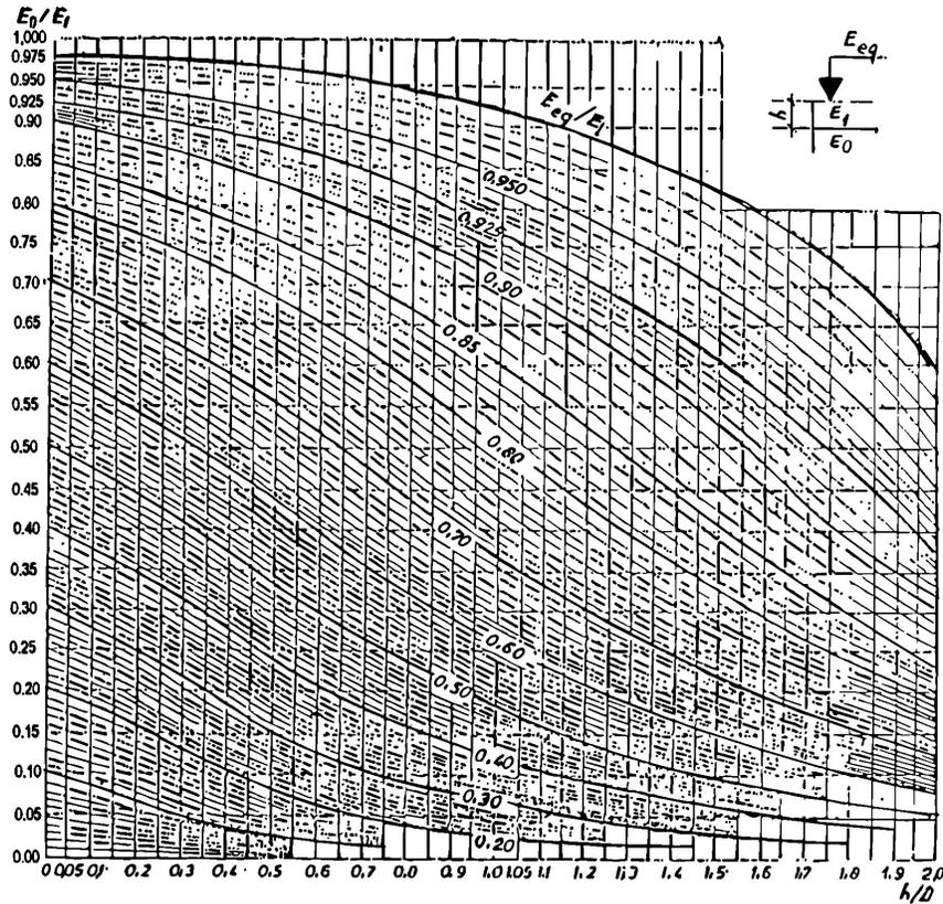
Fig. 8. Abacus for sizing flexible road systems
