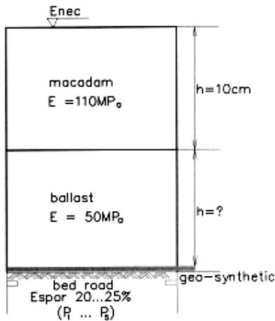
Fig. 7. The road system composed of a macadam and foundation of ballast placed on a geo-synthetic spread on the way bed
