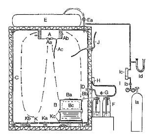
Fig. 1. Carbon dioxide generator [2]
