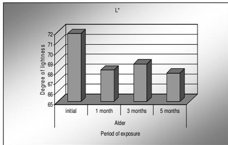
Fig. 6. Degree of lightness  $L^*$  recorded before and after the sunlight exposure for 1, 3 and 5 months, under indoor circumstances, behind a window glass for veneers made of black alder
