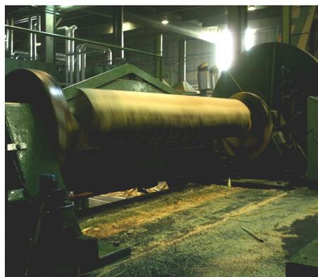
Fig. 1. *Half-rounded slicing method*
