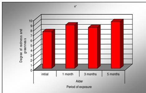
Fig. 7. Degree of redness and greenness  $a^*$  recorded before and after the sunlight exposure for 1, 3 and 5 months, under indoor circumstances, behind a window glass for veneers made of black alder
