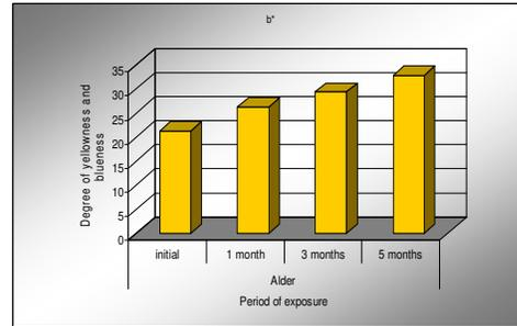
Fig. 8. Degree of yellowness and blueness  $b^*$  recorded before and after the sunlight exposure for 1, 3 and 5 months, under indoor circumstances, behind a window glass for veneers made of black alder
