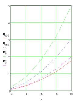
Fig. 5. The curvature radius in rapport with the velocity determined with different calculus relations
