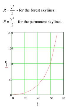
Fig. 4. The variation of the calculus error in function of the slope
