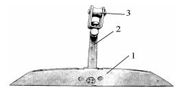
Fig. 1. A support for the main cable in case of the FP 2 skyline: 1 - blade; 2 - arm; 3 - catching system
