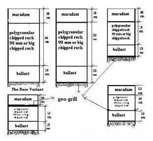
Fig. 1. Geo-grills in the road's structure
