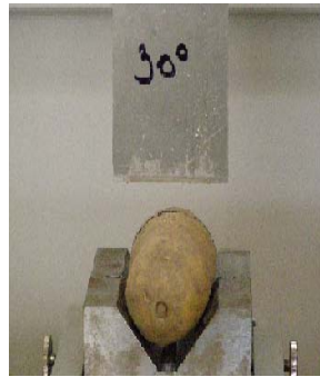
Fig. 5. The cutting knife with the sharpening angle of 30^\circ
