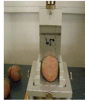
Fig. 6. The cutting knife with the sharpening angle of 45^\circ
