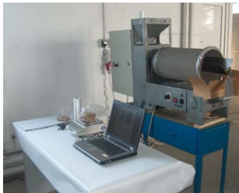
Fig. 1. Adapted stand for investigation of the cylinder separator working process
