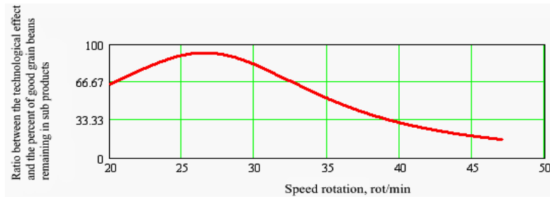
Fig. 7. Ratio variation between technological effect and the percent of good grain beans remaining in sub products depending to the cylinder separator speed rotation
