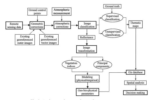
Fig. 2. A schematic diagram of general image processing procedures in remote sensing
