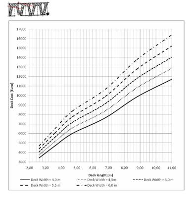
Fig. 2. Π-Beam deck costs, in function of width and length
