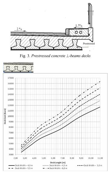
Fig. 4. The cost of  $\perp$ -beams decks, in function of width and length
