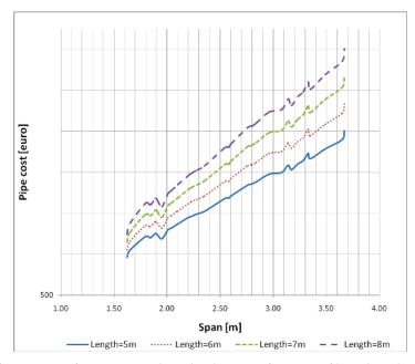
Fig. 9. Costs for corrugated steel culverts in function of length and span
