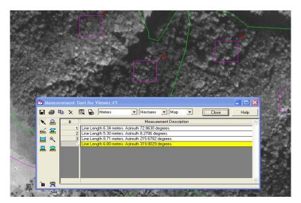
Fig. 2. Measuring the diameter using the "measure" command in ERDAS software
