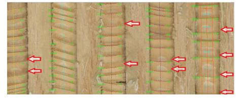
Fig.2. The detail of some WinDENDRO paths with growth rings measured on a fir compression wood sample (marked with arrow)
