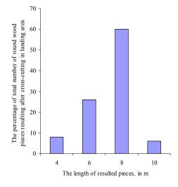
Fig. 2. The percentage of total number of round wood pieces resulting after cross-cutting in handing area
