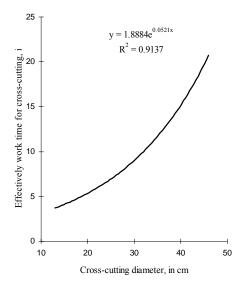
Fig. 7. Correlation between time for cross-cutting and diameter of cross-cutting
