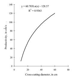
Fig. 8. Correlation between cross-cutting productivity and diameter of cross-cutting
