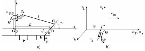
Fig. 1. *Kinematics of a point from the complex aggregate blade-bearing bar: a) the running mechanism; b) mobile and stationary reference*
