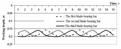
Fig. 5. The operation process executed by different blade types in a vertical plane
