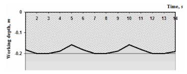
Fig. 4. The operation process executed by the blade in vertical plane
