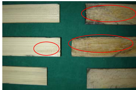
Fig. 5. Inner degradation of fir (left) and beech (right) revealed after slicing
