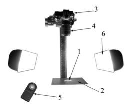
Fig. 4. Experimental stand used for the image acquisition of the seed probes: 1 – seed probe, 2 – lusterless black background for the attenuation of shadows, 3 – DSLR camera, 4 – lens system, 5 – infrared camera trigger, 6 – fluorescent light lamp.
