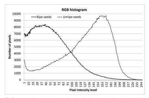
Fig.7. The RGB histogram analysis of seed quality based on pixel intensity level value.
