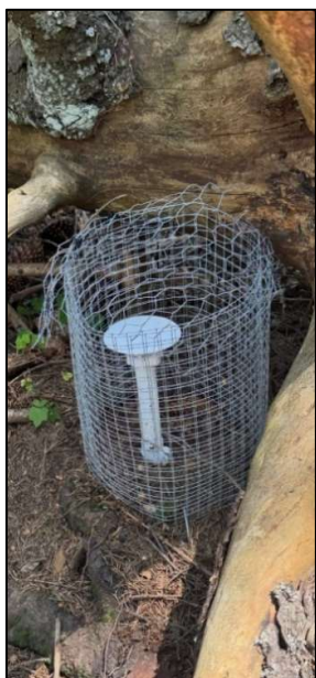
Fig. 2. A TMS-4 sensor installed in the study site covered with a wire mesh to protect from wildlife
