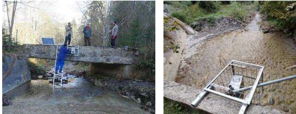
Fig. 2. Non-contact radar discharge sensor (Sommer RQ-30) installed above the stream at the Tigăi catchment site (Foto Mihalache A.)
