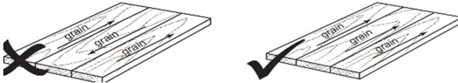
Fig. 3. Panel joined incorrectly and correctly joint solid timber [15]
