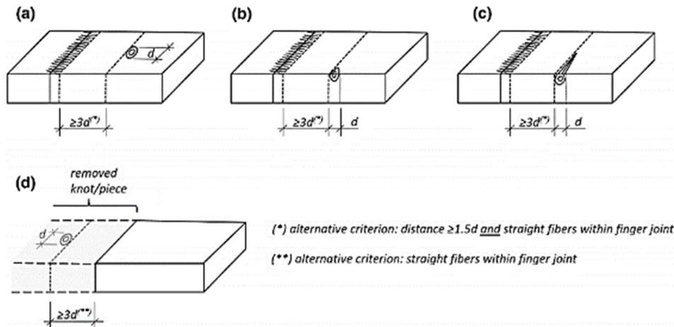
Fig. 2. Details of finger-jointed timber showing the minimum distance between knot and finger-joint in cases where the knot is [33]: a. a round knot (oval knot); b. an arris knot; c. a splay knot; d. a case where the knot is removed
