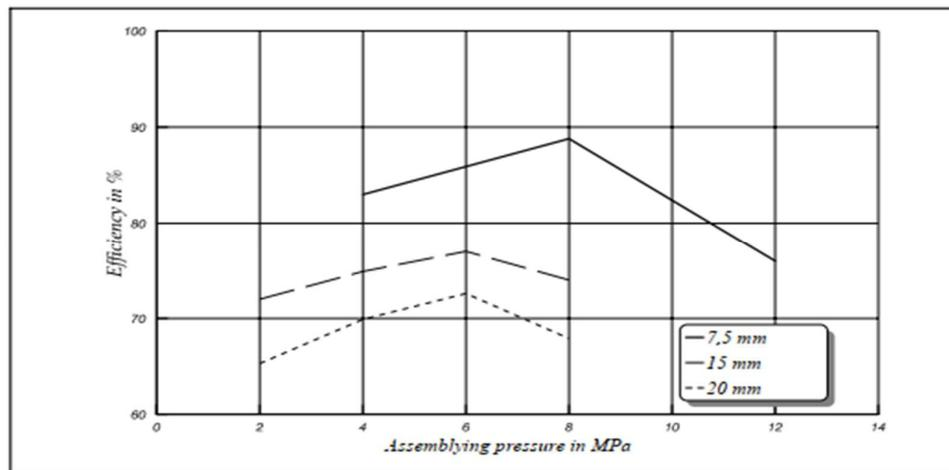
Fig. 1. Finger joint efficiency as a function of assembly pressure [12]
