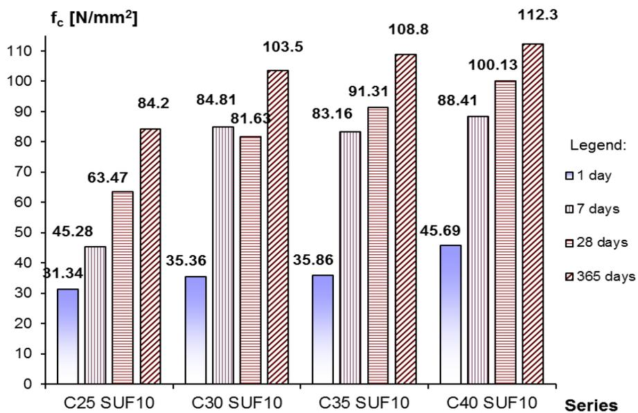
Fig. 3. Compressive strengths
