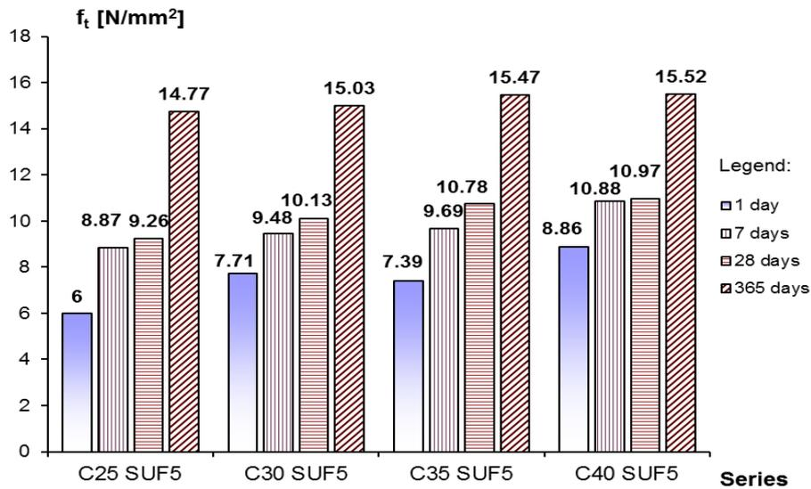
Fig. 2. Bending tensile strengths
