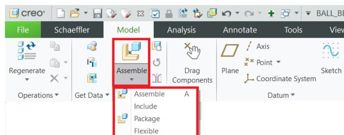
Fig. 4. Option for mounting assembly
