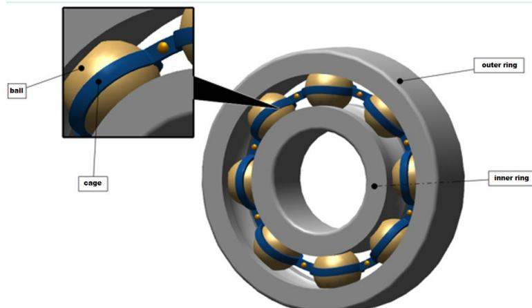
Fig. 3. *Illustration of the designed elements of the assembly*
