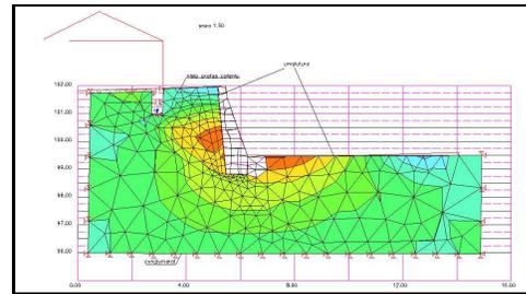
Fig. 14. *Chart of unitary horizontal efforts in work stage 3*
