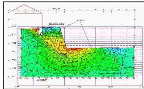
Fig. 10. Distribution of horizontal efforts in the ground next to the neighbouring building at the initial stage
