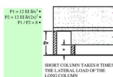
Fig. 2. The ratio between the forces applied to the short columns and long columns
