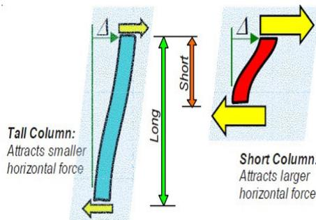
Fig. 4. *Short columns attracts shear forces more than the tall columns [2]*
