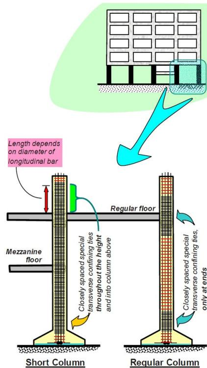
Fig. 8. Reinforcement details [1]
