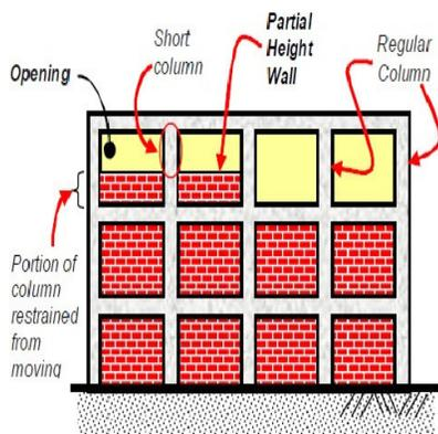
Fig. 7. Walls with short columns and long columns at the same level [2]
