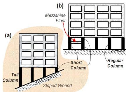
Fig. 1. Building with short columns [2]
