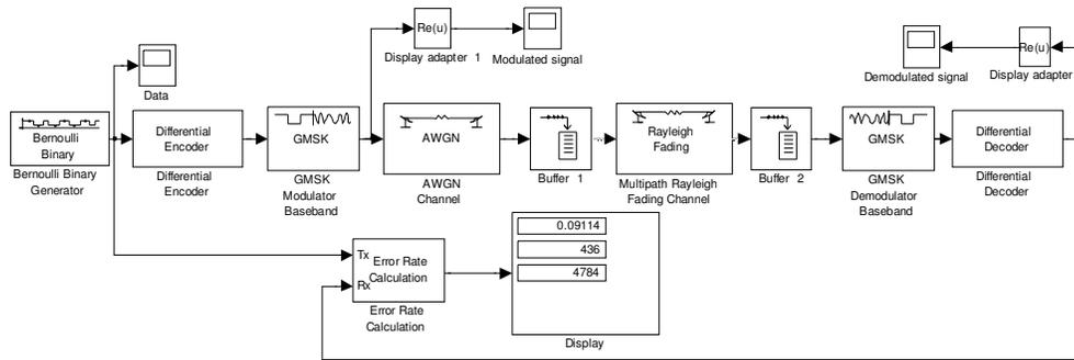
Fig. 1. Complete GSM Simulation model
