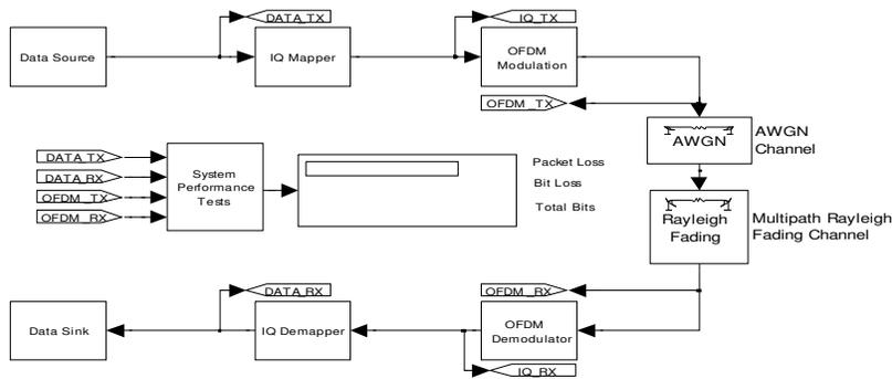
Fig. 2. Complete OFDM Simulation model
